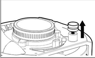
1. Pull the pin to unlock the door.
