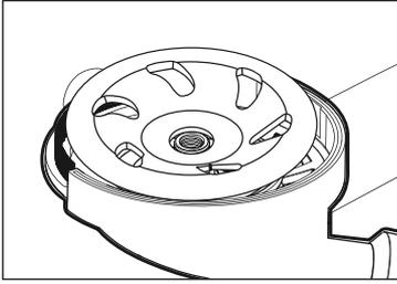
4. Install cup wheel onto grinder shaft. Ensure cup wheel does not contact shroud.
