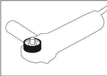
1. If grinder guard neck on gear casing neck is too small, use adapter bushing so shroud fits tightly.
