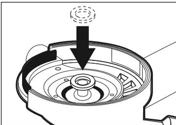
3. Smaller shim is for use with grinders that have a 5/8" shaft, to extend the cup wheel.
