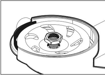
5. Screw grinder flange nut if needed on 7/8" arbor cup wheels.
