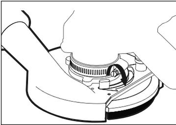
6. Tighten hose clamp so shroud is firmly attached to grinder. Cup wheel should extend past shroud approximately 1/16".
