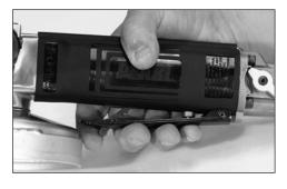
4. Use the lever to control air flow. Begin grinding.
