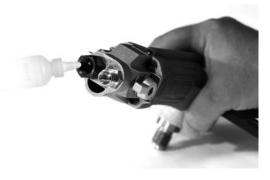
Grease gears as needed using a multi-purpose EP lithium grease or moly EP lithium grease. DO NOT use oil.
