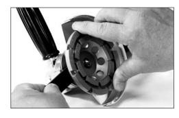
2. Screw on cup wheel and tighten.
