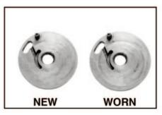
Wear in rear plate due to worn bearings.
