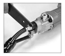
3. Tighten the air hose nut.
