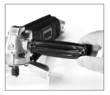
9. Attach the handle and tighten.
