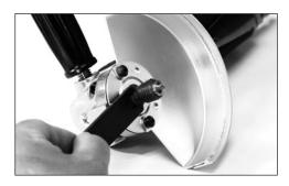
1. Place wrench on bottom of spindle.
