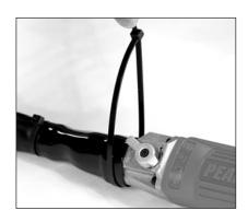
7. Use the fastener to secure exhaust hose to the grinder.
