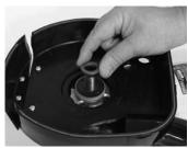
6. Place washer on top of cup nut as needed.
