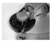
5. Tighten hose clamp so shroud is firmly attached to grinder.
