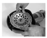
7. Once shroud is tightly attached to the grinder, attach cup wheel as normal. Ensure cup wheel does not contact shroud.
