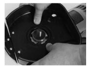
4. Push and twist until shroud Interior O-ring snaps into spacer exterior groove.
