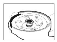
4. Screw grinder flange nut if needed on 7/8" arbor cup wheels.
