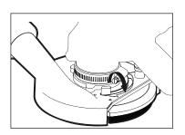
5. Tighten hose clamp so shroud is firmly attached to grinder. Cup wheel should extend past shroud approximately 1/16".
