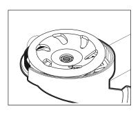
Install cup wheel onto grinder shaft. Ensure cup wheel does not contact shroud.
