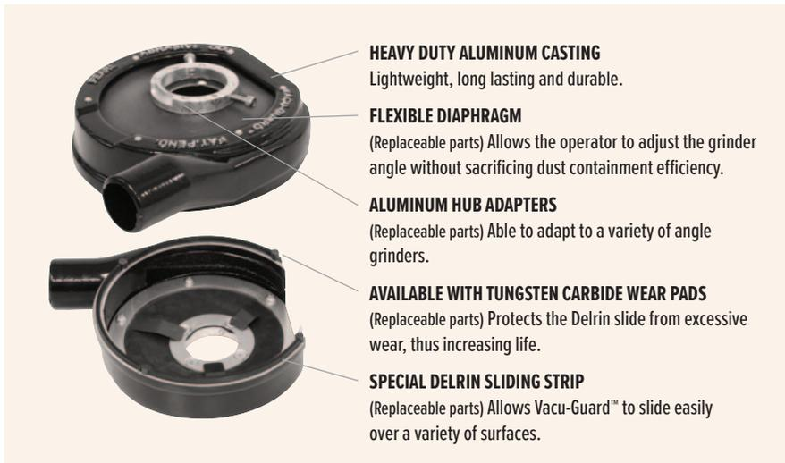
Designed to fit the following 4-1/2" and 7" grinders: Black & Decker, Bosch, Makita, Metabo, Dewalt, Milwaukee, Hitachi
